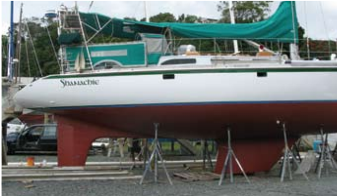
≈ ABOVE: Exterior views of Shanachie during various haul-outs, showing keel, rudder, and skag configurations, stern scoop, cockpit, and travel-lift positioning, with bow thruster visible in lower right photo.
