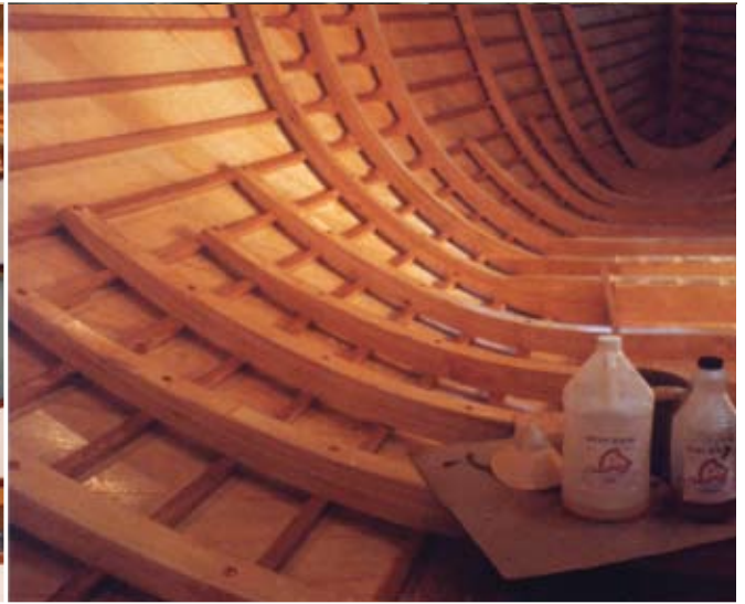
≈ Views of Shanachie's various construction stages, her laminated beams, the under-floor mast step, and original lines by New Zealand designer Paul Whiting, below.
